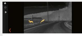
□ BMW Night Vision<sup>1</sup> with person recognition makes people and large animals visible on the Control Display from a distance using heat imaging and illuminates them with the Dynamic Marker Light in the main headlight. An additional warning system is also automatically activated when the vehicle is started, regardless of the status of the imaging display.
