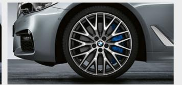
O 20" light alloy wheels Cross-spoke style 636 in Bicolor Orbit Grey, bright turned on the visible side. TPMS complete wheel set with run-flat mixed tyres, wheel size 8J x 20 and 9J x 20.
