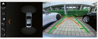
□ The Rear view camera<sup>7</sup> enables improved orientation when reversing at speeds below 15 km/h, for example when parking. It shows the area behind the car on the Control Display. Interactive track lines for measuring distance and turning circles assist the driver when manoeuvring, obstacles are marked in colour.
