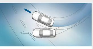
■ Dynamic Stability Control (DSC) permanently assesses the vehicle's movements and stabilises it using engine and braking regulation when unstable driving conditions are detected. Additional features of DSC are, for example, brake drying, braking readiness or the Hill-Start assistant, which holds the vehicle briefly in place when starting on inclines to prevent it from rolling backwards.
