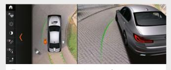
□ The equipment package Parking Assistant Plus<sup>7</sup> makes parking and manoeuvring the vehicle easier. It features Surround View including Top View, Remote 3D View, PDC and the Parking Assistant with linear guidance, which parks the vehicle parallel or perpendicular to the lane completely automatically. The system works by measuring potential spaces while driving past them at a low speed.
