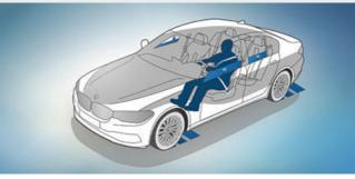
□ Active Protection is the BMW ConnectedDrive preventive passenger protection system. Active Protection warns the driver if it detects signs of tiredness, safety belts are pretensioned in critical situations, electric seats are returned to upright positions and the windows and sliding roof are closed. After an accident occurs, the brakes are automatically applied until the vehicle reaches a standstill.
