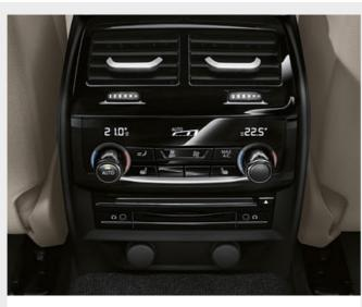
□ The Automatic air conditioning with 4-zone control comes with the equipment included in Automatic air conditioning with 2-zone control with extended features, along with two air vents in the B columns. Additionally, the rear passengers can individually adjust their own climate via a separate control element with display.
