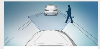
■ Person warning with light city braking function<sup>2</sup> actively assists the driver with the prevention of collisions involving pedestrians. It is active at speeds of up to 60 km/h and preconditions the brakes for increased responsiveness. In the event of an emergency, the system prevents a collision or ensures that the collision speed is reduced considerably.
