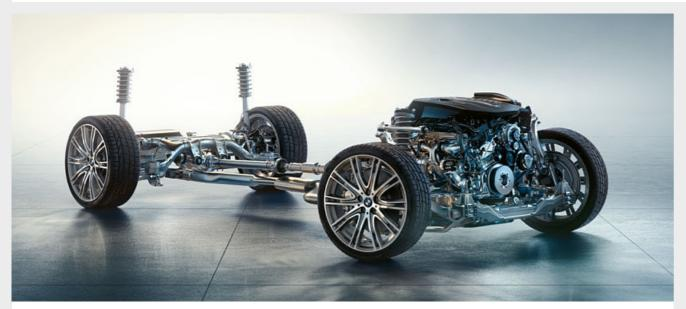
**Integral Active Steering**<sup>1, 5</sup> combines support that varies based on the steering angle on the front axle, and rear wheels that also contribute to steering. At lower speeds, it offers greater manoeuvrability and agility by turning the rear wheels opposite the front wheels. Beginning around 60 km/h, the rear wheels turn parallel to the front wheels, to increase driving stability and comfort.
