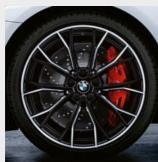
O 20" M light alloy Double-spoke style 669 M wheels, Bicolour with mixed tyres and runflat properties, front wheel size 8J x 20 with tyres 245/35 R20, rear wheel size 9J x 20 with tyres 275/30 R20.
